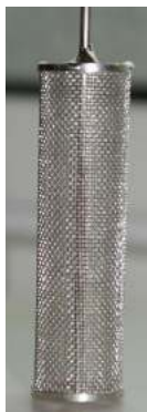
Figure 11.3.3 . Example of a cylindrical Pt-gauze electrode used in controlled-potential coulometry. The electrode shown here has a diameter of 13 mm and a height of 48 mm, and was fashioned from Pt wire with a diameter of approximately 0.15 mm. The electrode's surface has 360 openings/cm 2 and a total surface area of approximately 40 cm 2 .
