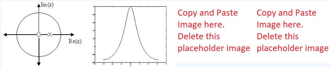
Figure 11.9.2: The (a) Pole/Zero Plot figure represents the pole/zero plot while the Frequency Response ( |H(w)| ) shows the frequency response with a peak at +2 and graphed between plus and minus \pi .
