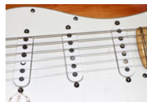
Figure 10.2.3 : Pickups on an electric guitar.
