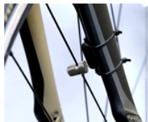
Figure 10.2.4 : Bicycle computer sensor and magnet.
