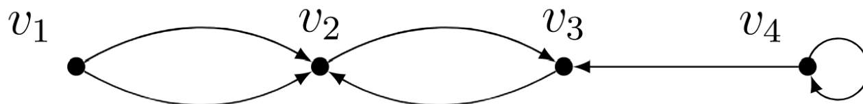
Figure 14.3.1: Diagram of the directed graph G = (V, E) .
