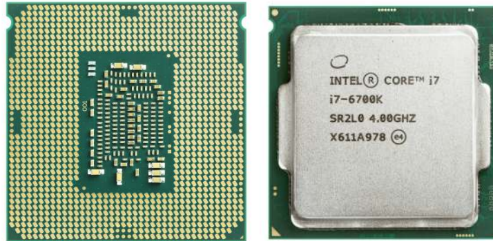
Figure 2.2.2: (a) Bottom view of an Intel central processing unit Core i7 Skylake type core, model 6700K. LGA 1151 socket, 14 nm process, core frequency 4.00 GHz. Manufactured in Vietnam. Image by Eric Gaba is licensed under CC BY-SA . (b) Top view of an Intel central processing unit Core i7 Skylake type core, model 6700K. LGA 1151 socket, 14 nm process, core frequency 4.00 GHz. Manufactured in Vietnam. Image by Eric Gaba is licensed under CC BY-SA
