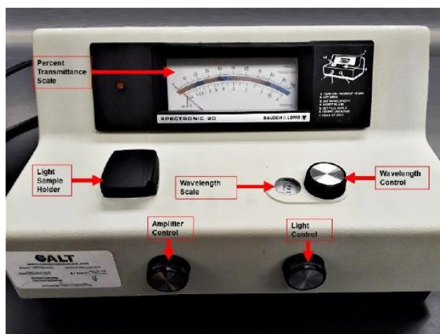
Figure 2. Labeled parts of a spectrophotometer
