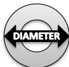
Figure 2. diameter of washer, measured in a straight line across the center of the washer from outer edge to outer edge.
