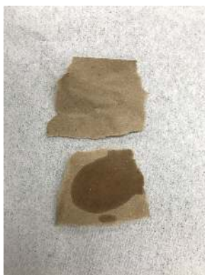
Figure 8. Negative grease spot test (left) and positive grease spot test (right). (original photo)
