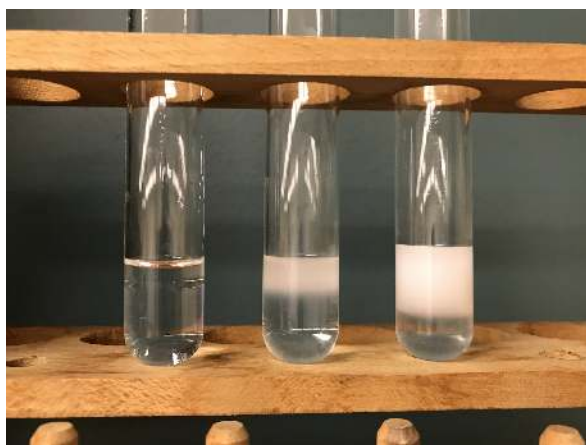
Figure 7. Negative ethanol emulsion test (left) and positive ethanol emulsion test (right two tubes). (original photo)
