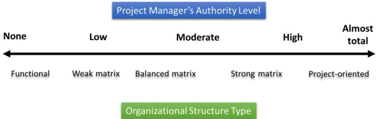
Figure 2.5: The Spectrum of Organizational Structure Types based on Project Manager’s Authority Level
