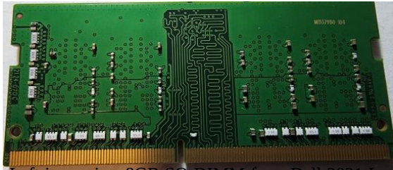
Figure 2.3.5: Left image is a 8GB SO-DIMM for a Dell 2021 Laptop. Right image is 16GB SO-DIMM for a Dell 2021 Laptop. Images by Ly-Huong Pham, is licensed CC BY-NC-SA
