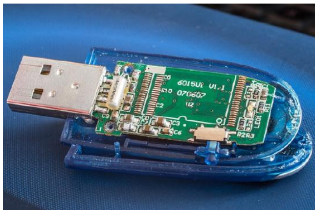
Figure 2.4.1: Left image is an inside view of an USB. Image by Silke from Pixabay, is licensed CC BY; The right image is USB Connections. Image by Bruno /Germany is licensed CC BY-SA 2.0
