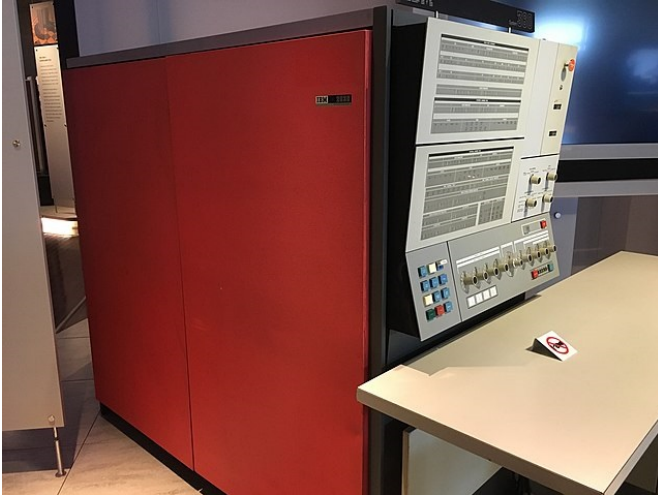
Figure 1.3.4 IBM System/360 Model 30 central processor unit (CPU). Image by Arnold Reinhold is licensed CC BY-SA 3.0 (opens in new window)
