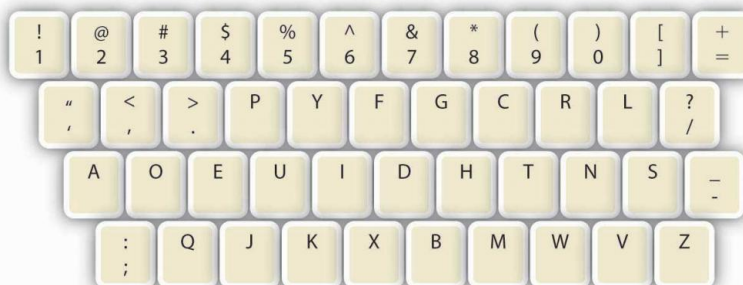
Figure 12.1.11: The Dvorak keyboard is a more efficient design compared to the QWERTY keyboard. Due to resistance from typists, manufacturers, and teachers, it never gained widespread adoption.
