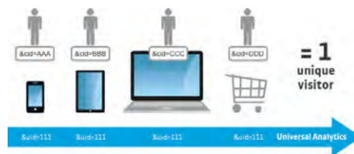
Figure 7.3.3: Universal Analytics can now track individual users across devices and touchpoints Adapted From Treefish, n.d.
