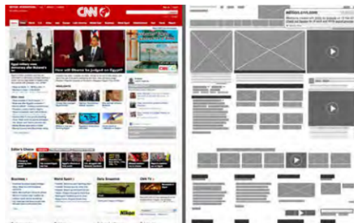
Figure 6.5.3: An example of a wireframe against what the final website looks like Adapted From Wirify, 2017
