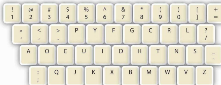
Figure 14.3.11: The Dvorak keyboard is a more efficient design compared to the QWERTY keyboard. Due to resistance from typists, manufacturers, and teachers, it never gained widespread adoption.
