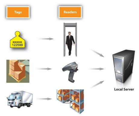
Figure 9.8: How RFID Tagging Works. Some consumer groups worry that RFID tags and electronic product codes could be used to track their consumption patterns or for the wrong purposes. But keep in mind that like your car-door remote, the codes and tags are designed to work only within short ranges. (You know that if you try to unlock your car from a mile away using such a device, it won't work.)
