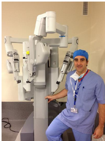
Figure 11.14: Intuitive Surgical is the maker of the da Vinci robot, a new type of technology used to make surgeries easy to perform and less invasive. Intuitive Surgical often demonstrates the robot at surgical conventions. Docor Comunicacion – Da Vinci robot – CC BY-NC-ND 2.0.
