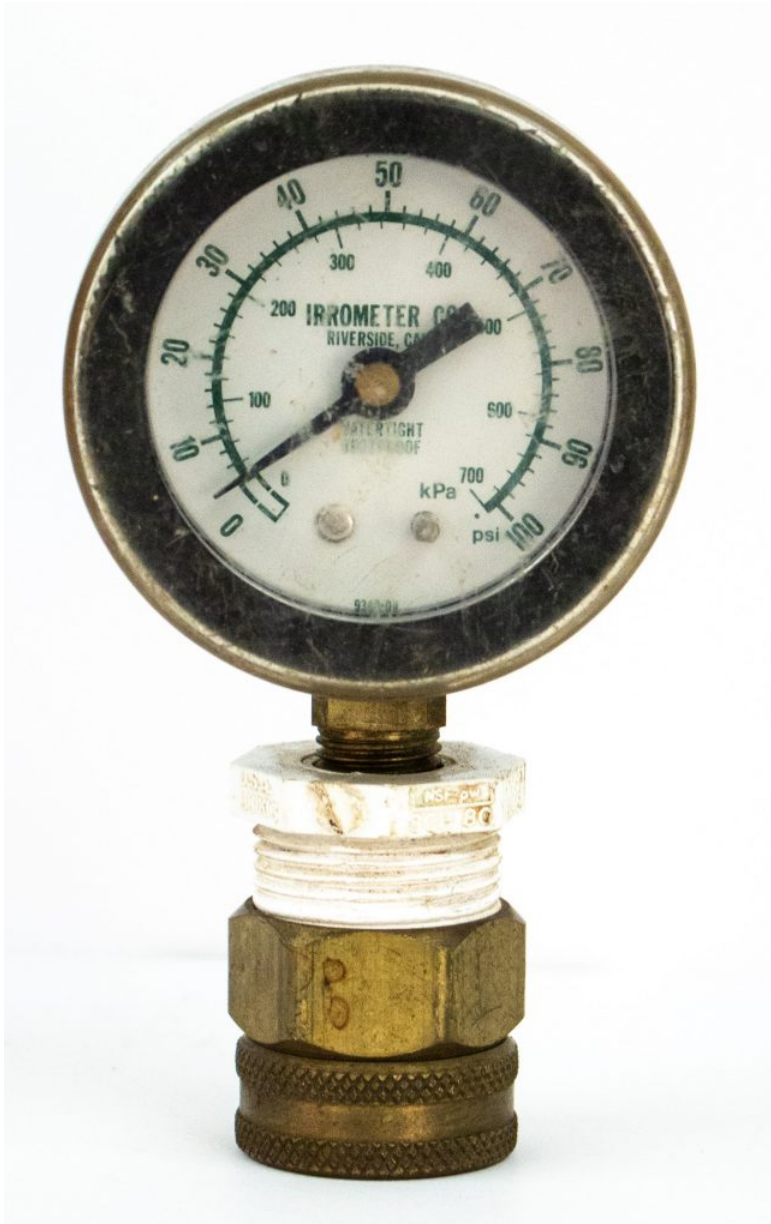
Water Pressure Test Gauge by Gwen Arkin is licensed under CC BY 4.0
