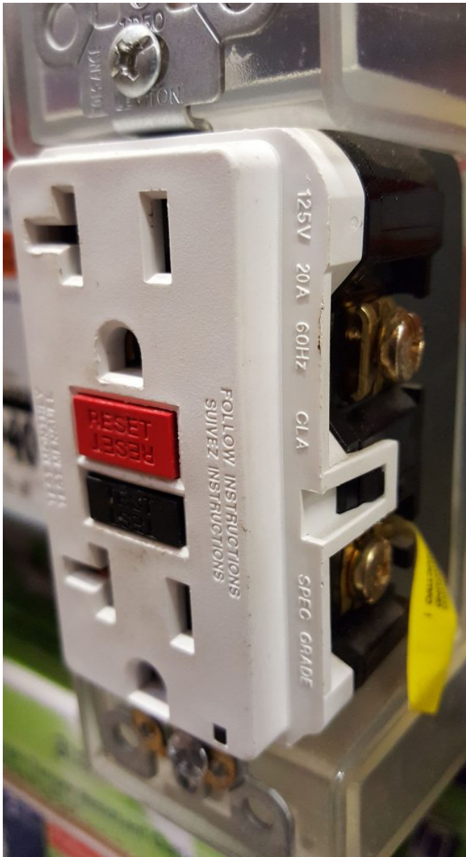
GFCI Receptacle by Clifford Rutherford is licensed under CC BY 4.0
