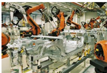
Figure 9.6: Robots at work in a BMW factory in Leipzig, Germany
