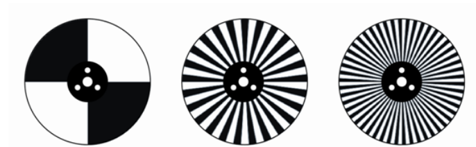
Figure 6.3B.11. Illustration of several chopper designs.
