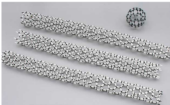
Figure 2.8b Fullerene (upper right) and tubes of rolled up graphenes (lower three).
