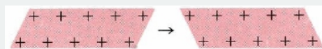
Figure 16.4.3: Malleability of metals originates from each of moving layers of atoms with respect to each other. The final situation is much the same as the initial. Thus if we hit a metal with a hammer, the crystals do not shatter, but merely change their shape. This is very different from the behavior of ionic crystals.
