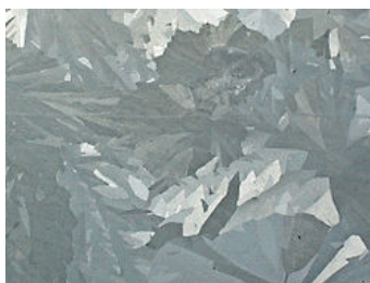
Crystalline surface of a hot-dip galvanized steel surface. This served both as prophylactic protection (protecting the underlying steel from the oxygen in the air) and cathodic protection (once exposed, the zinc will oxidize before the underlying steel).
