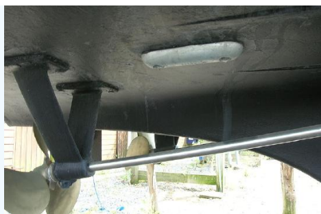
Zinc sacrificial anode (rounded object screwed to underside of hull) used to prevent corrosion on the screw in a boat via cathodic protection. Image by Rémi Kaupp and used with permission.
