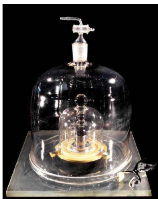
Figure 1.4.1: The Kilogram. The standard for the kilogram is a platinum-iridium cylinder kept in a special vault in France. Source: Photo reproduced by permission of the Bureau International des Poids et Mesures, who retain full internationally protected copyright.
