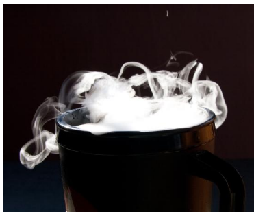
Dry ice ( \text{CO}_2(\text{s}) ) sublimed in air under room temperature and pressure. from Wikipedia.
