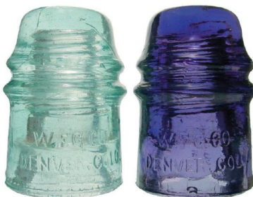
Figure 20.7.1: Radiation Damage. When high-energy particles emitted by radioactive decay interact with matter, they can break bonds or ionize molecules, resulting in changes in physical properties such as ductility or color. The glass electrical insulator on the left has not been exposed to radiation, but the insulator on the right has received intense radiation doses over a long period of time. Radiation damage changed the chemical structure of the glass, causing it to become bright blue. (CC BY-SA-NC; anonymous)
