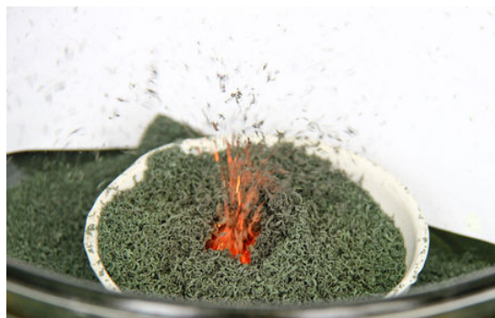
Figure 1: An Ammonium Dichromate Volcano: Change during a Chemical Reaction. The starting material is solid ammonium dichromate. A chemical reaction transforms it to solid chromium(III) oxide, depicted showing a portion of its chained structure, nitrogen gas, and water vapor (in addition, energy in the form of heat and light is released). During the reaction, the distribution of atoms changes, but the number of atoms of each element does not change. Because the numbers of each type of atom are the same in the reactants and the products, the chemical equation is balanced. (CC BY-SA 3.0; Mikk Mihkel Vaabel via Wikipedia). See video here: www.youtube.com/watch?v=CW4hN0dYnkM
