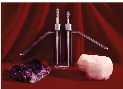
Figure 18.13.1 Isolation of Elemental Fluorine. The French chemist Henri Moissan was the first person to isolate elemental fluorine. A reproduction of the U-shaped electrolysis cell with which Moissan first isolated elemental fluorine in 1866 is shown with samples of cryolite (left) and fluorspar (right). Fluorspar is the raw material from which anhydrous hydrofluoric acid (HF) is prepared. Cryolite is a rare mineral that contains the fluoride ion.
