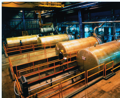
Figure 5.7.2: A Portion of a Plant for Separating Uranium Isotopes by Effusion of \text{UF}_6 . The large cylindrical objects (note the human for scale) are so-called diffuser (actually effuser) units, in which gaseous \text{UF}_6 is pumped through a porous barrier to partially separate the isotopes. The \text{UF}_6 must be passed through multiple units to become substantially enriched in ^{235}\text{U} .
