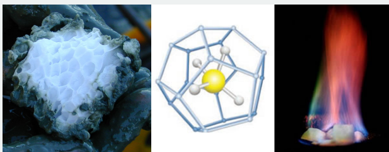
Figure 18.14.2: “Burning snowballs.” Like xenon, methane (CH 4 ) forms a crystalline clathrate with water: methane hydrate. When the solid is warmed, methane is released and can be ignited to give what appears to be burning snow. (left) Structure of a gas hydrate (methane clathrate) block embedded in the sediment of hydrate ridge, off Oregon, USA (CC-SA-BY-3.0 Wusel007 ) (middle) A ball-and-stick model of methane hydrate showing the central methane molecule surrounded by a “cage” of water molecules. Other hydrocarbon molecules such as pentane and ethane can occupy the central position in this structure. (United States Department of Energy image). (Right): A burning specimen of methane hydrate ice (United States Geological Survey image).
