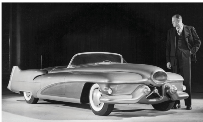
Figure 18.4.1: Magnesium Alloys Are Lightweight and Corrosion Resistant. Because magnesium is about five times lighter than steel and 50% lighter than aluminum, it was long considered the “material of the future,” as shown in this 1950 concept Buick LeSabre sports car made almost entirely of magnesium and aluminum alloys. Modern aluminum alloys usually contain about 5% magnesium to improve their corrosion resistance and mechanical properties.
