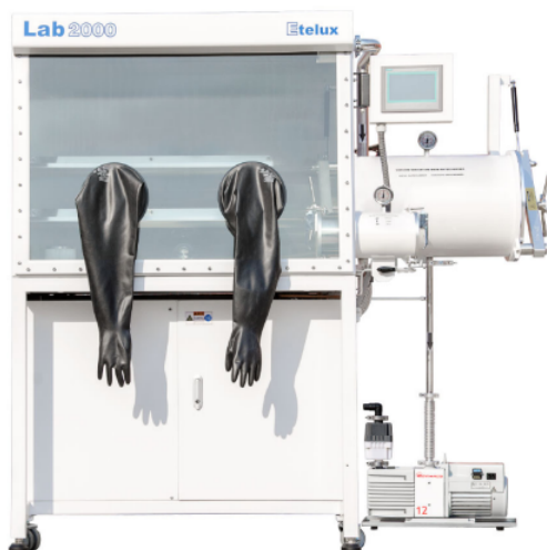
Figure 2: An inert-atmosphere glove box (reproduced from https://www.etelux-glovebox.com/prod...x-atmospheres/ )
