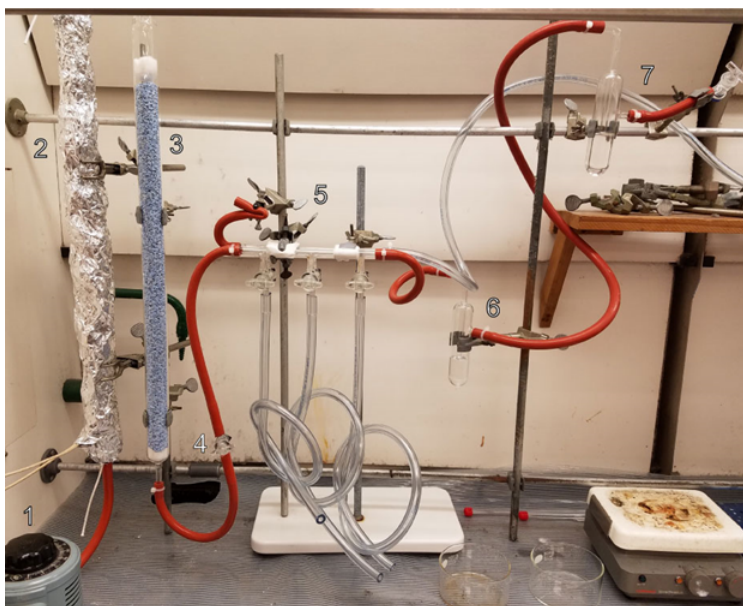
Figure 1 - Alane Schlenk Diagram. 1) Rheostat for heating element 2) oxygen scraper 3) drying column 4) valve to isolate columns 5) three-valve Schlenk manifold 6) first bubbler 7) second bubbler and final N 2 valve. Clear hose on the right connects to solvent trap for vacuum line.
