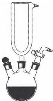
Figure 8-1 Three-neck flask equipped with a dry ice condenser.
