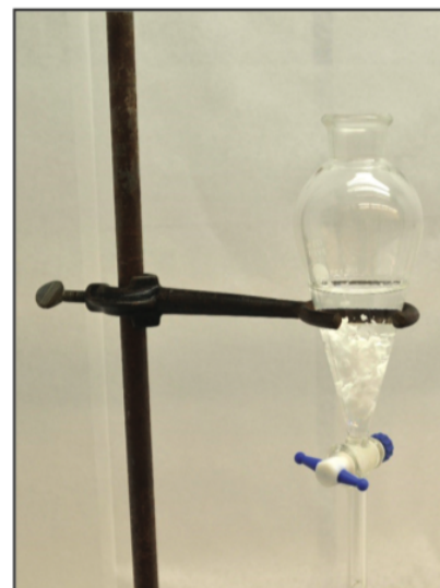
Figure 2.5. Adding HCl to the basic, aqueous phase leads to precipitation of benzoic acid, here seen as a white precipitate.
