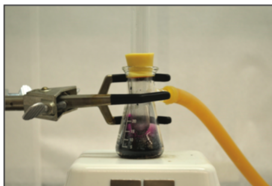
(B) The filter flask is heated. The crude material starts to sublime. Notice the rising purple vapor.
