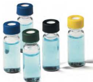
Figure 2.6: Appearance of HPLC/CE vials. The HPLC can also use plastic vials that look quite similar. Image is taken from www.thermofisher.com
