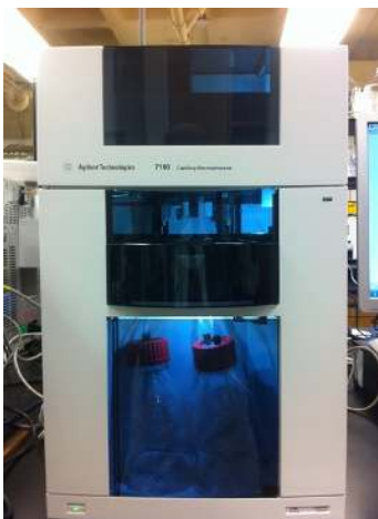
Figure 6.7: Agilent Technologies 7100 Capillary Electrophoresis, UCD Capillary Electrophoresis instrument. Note that multiple vials can be probed sequentially if required. This instrument is located in room 3475.
