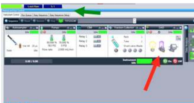
Figure 2.5: "Instrument Control" tab indicated by top, green arrow. Bottom right, red arrow indicates the DAD window.
