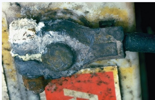
Corroded battery terminals. The white solid is lead(II) sulfate, formed from the reaction of solid lead with a solution of sulfuric acid.
