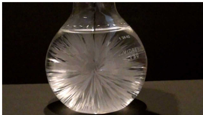
Figure 1.3.4: The Crystallization of Sodium Acetate from a Concentrated Solution of Sodium Acetate in Water. The addition of a small “seed” crystal (a) causes the compound to form white crystals, which grow and eventually occupy most of the flask. Video can be found here: https://www.youtube.com/watch?v=BLq5NibwV5g
