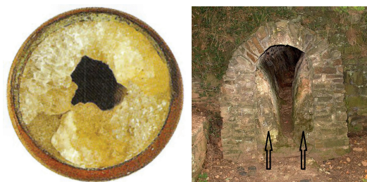
Figure 3: Calcium carbonate deposits (left) Calcium carbonate ( \text{CaCO}_3 ) deposits in hot water pipes can significantly reduce pipe capacity. These deposits, called boiler scale, form when dissolved \text{CO}_2 is driven into the gas phase at high temperatures. (right) Highly calcified remains of Eifel aqueduct near Euskirchen-Kreuzweingarten, Germany. Figure used with permission from Wikipedia
