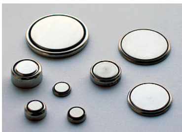
Button batteries. Photo courtesy of Gerhard H Wrodnigg, Images used with permission from Wikipedia
