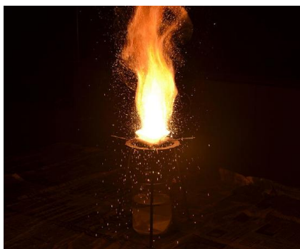
Figure 7.6.3: The thermite reaction produces so much heat that the iron it produces comes out molten, a property that makes this reaction useful in welding. Image by Kingfisher [CC BY-SA 3.0 ( https://creativecommons.org/licenses/by-sa/3.0 )], from Wikimedia Commons.
