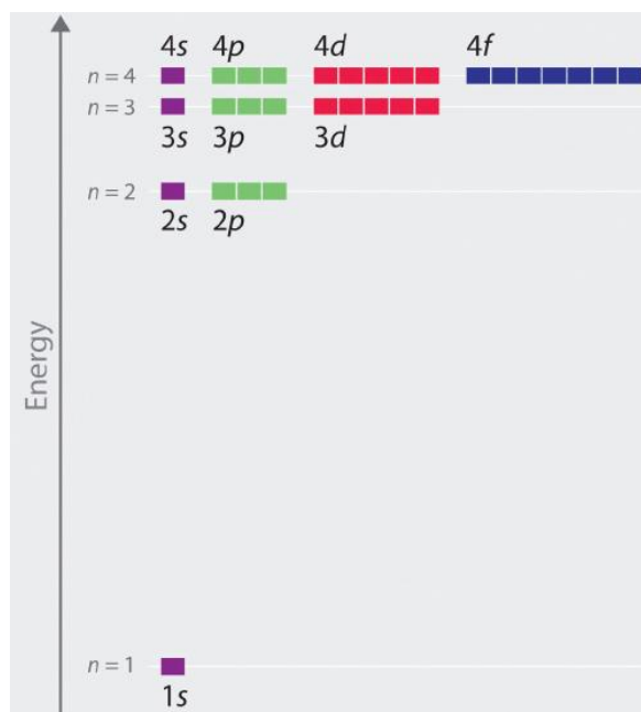
Figure 6: Orbital Energy Level Diagram for the Hydrogen Atom with a single electron. Each box corresponds to one orbital. Note that the difference in energy between orbitals decreases rapidly with increasing values of n .
