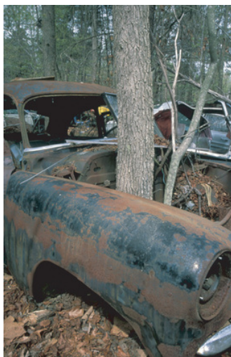
Figure 9.1.2: Rust Formation. The corrosion process involves an oxidation–reduction reaction in which metallic iron is converted to \text{Fe}(\text{OH})_3 , a reddish-brown solid.
