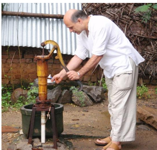
Figure 4.8.1: The manual water pump draws water up from a well by creating a vacuum that water rushes in to fill. Hand pump to pump water from a well in a village near Chennai in India. Image used with permission (CC BY 2.0; Sustainable Sanitation Alliance ).
