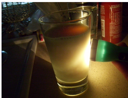
Figure 1: Tyndall Effect, the Scattering of Light by Colloids
