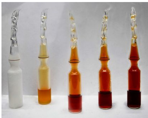
Figure 7.1.1: Dinitrogen tetroxide is a powerful oxidizer that reacts spontaneously upon contact with various forms of hydrazine, which makes the pair a popular propellant combination for rockets. Nitrogen dioxide at -196\text{ }^{\circ}\text{C} , 0\text{ }^{\circ}\text{C} , 23\text{ }^{\circ}\text{C} , 35\text{ }^{\circ}\text{C} , and 50\text{ }^{\circ}\text{C} . ( \text{NO}_2 ) converts to the colorless dinitrogen tetroxide ( \text{N}_2\text{O}_4 ) at low temperatures, and reverts to \text{NO}_2 at higher temperatures. Figure used with permission from Wikipedia (CC BY-SA 3.0; Eframgoldberg ).
