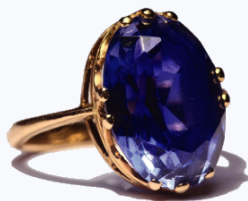
Figure 4: Although pure aluminum oxide is colorless, trace amounts of iron and titanium give blue sapphire its characteristic color. (credit: modification of work by Stanislav Doronenko)
