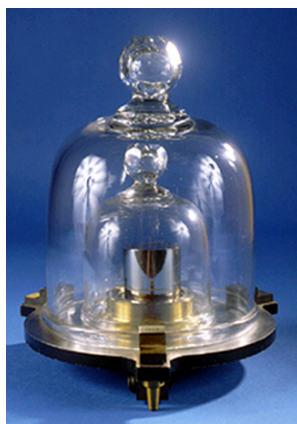
Figure 1.5.2: This replica prototype kilogram is housed at the National Institute of Standards and Technology (NIST) in Maryland. (credit: National Institutes of Standards and Technology).
