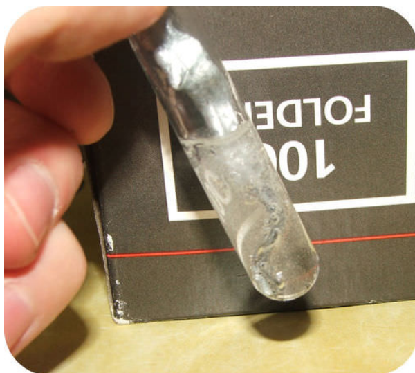
Figure 11.3.1: Zinc metal reacts with hydrochloric acid to give off hydrogen gas in a single-replacement reaction.
