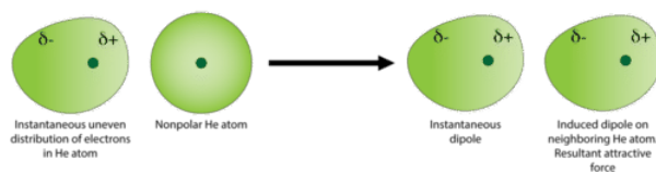
Figure 5.3.9: Random fluctuations in the electron density within the electron cloud of a helium atom results in a short-lived ("instantaneous") dipole. The attractive force between instantaneous dipoles and the resulting induced dipoles in neighboring molecules is called the London dispersion force.
