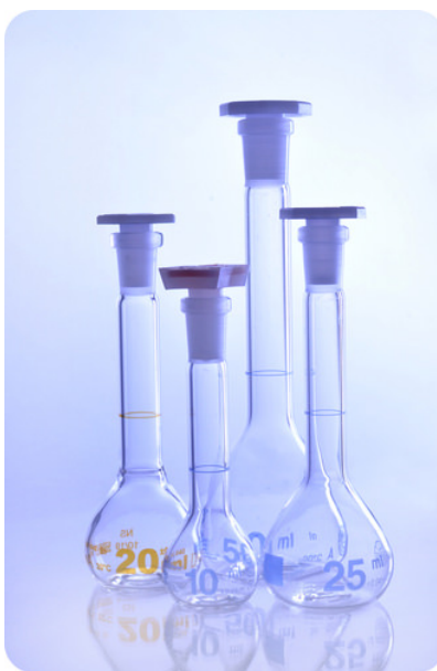
Figure 8.1.3: Volumetric flasks come in many sizes, each designed to prepare a different volume of solution.
