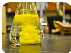
Figure 10.4.6: A yellow precipitate of solid lead (II) iodide forms immediately when solutions of lead (II) nitrate and potassium iodide are mixed.
