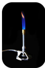
Figure 10.5.2 A Bunsen burner is commonly used to heat substances in a chemistry lab. Methane is reacted with oxygen to form carbon dioxide and water.
