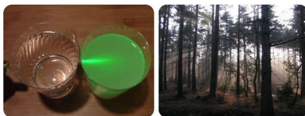
Figure 7.6.2: Light passes through a colorless solution and is not scattered. When it passes through a diluted milk solution, the light is scattered by colloidal particles, an observation of the Tyndall effect. The Tyndall effect allows sunlight to be seen as it passes through a fine mist.
