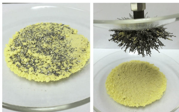
Figure 2.2.4: Iron and sulfur as a mixture (left) and separated by physical means (right).
