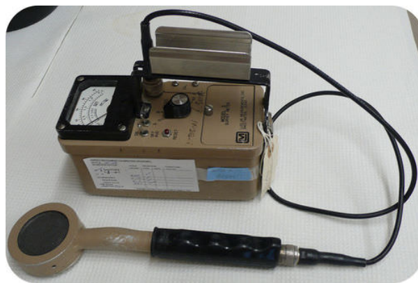
Figure 10.2.4: A Geiger counter is used to detect radiation.
