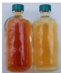
Figure 3.1.2: \text{NO}_2 (left) is a reddish-brown toxic gas that is a prominent air pollutant produced by internal combustion engines. It is converted to \text{N}_2\text{O} (right) at low temperatures.
