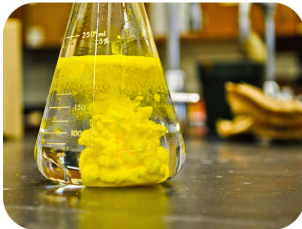
Figure 11.3.3: When a few drops of lead (II) nitrate are added to a solution of potassium iodide, a yellow precipitate of lead (II) iodide immediately forms in a double-replacement reaction.
