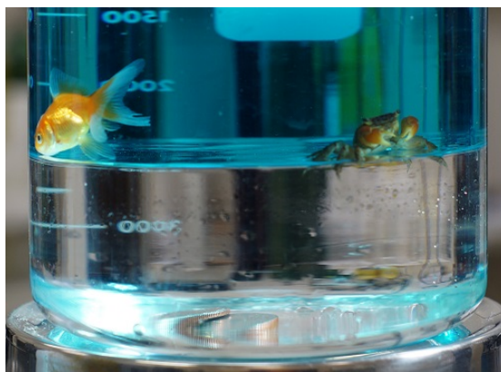
Figure 9.1.1: A beaker holds water with blue food dye (upper liquid layer) and a much more dense perfluoroheptane (a fluorocarbon) lower liquid layer. The two fluids cannot mix and the dye cannot dissolve in fluorocarbon. A goldfish and a crab have been introduced into the water. The goldfish cannot penetrate the dense fluorocarbon. The crab floats at the liquid boundary with only parts of his legs penetrating the fluorocarbon fluid, unable to sink to the bottom of the beaker. Quarter coins rest on the bottom of the beaker. Animals were rescued from their predicament after the photo was taken. Figure used with permission from Wikipedia (Sbharris (Steven B. Harris)).
