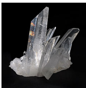
Figure 8.2.1: Crystalline Arrangement of Quartz crystal cluster. Some large crystals look the way they do because of the regular arrangement of atoms (ions) in their crystal structure. from Wikipedia.
