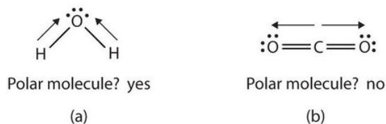
Figure 4.4.7 Physical Properties and Polarity. The physical properties of water and carbon dioxide are affected by their polarities.
