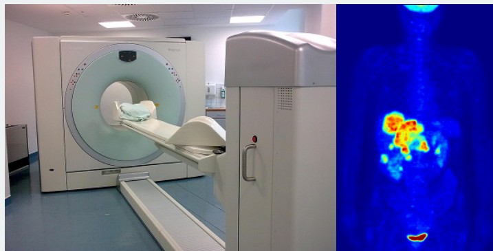
Figure 11.4.3: (left) Combined apparatus for positron emission tomography (PET) and X-ray computer tomography (CT), Siemens Biograph (right) Whole-body PET scan using ^{18}\text{F} -FDG. Images used with permission from Wikipedia.
