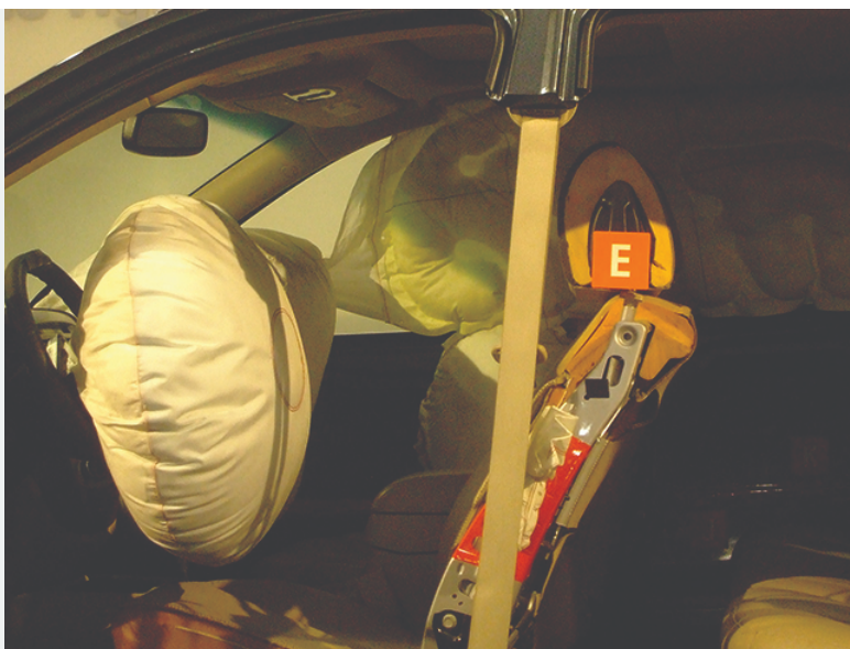
Figure 8.4.3: Airbags deploy upon impact to minimize serious injuries to passengers. (credit: Jon Seidman)
