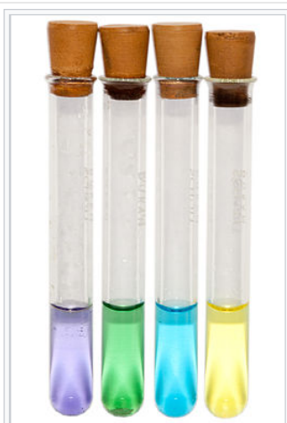
From left: [V(H_2O)_6]^{2+} (lilac), [V(H_2O)_6]^{3+} (green), [VO(H_2O)_5]^{2+} (blue) and [VO(H_2O)_5]^{3+} (yellow).
