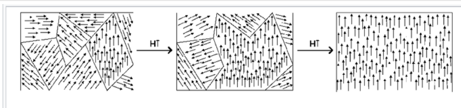
Rotation of orientation and increase in size of magnetic domains in response to an externally applied magnetic field.
