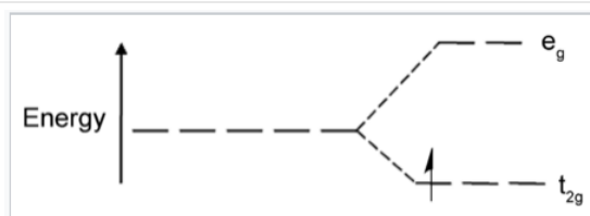
Crystal field energy diagram for the d^1 octahedral complex [\text{Ti}(\text{H}_2\text{O})_6]^{3+} .
