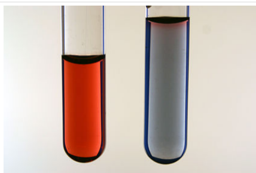
Aggregation of Au nanoparticles (in this case by adding salt to a colloidal solution) causes a color change from wine red (left) to blue (right). Photo credit: George Lisensky, Beloit College
