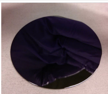
A 2" wafer cut from a GaAs single crystal. GaAs, like many p-block semiconductors, has the zincblende structure.
