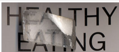
Calcite crystals are birefringent, meaning that their refractive indices are different along the two principal crystal directions. This gives rise to the phenomenon of double refraction.
