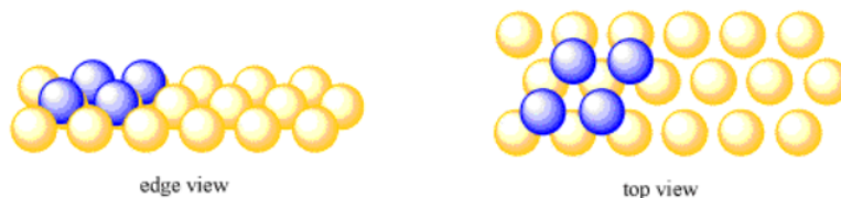
Figure 2.3.6: Adding a second layer of atoms to a hexagonal layer.
