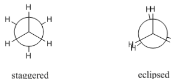
Figure 6.2.7: Newman projections showing staggered (left) and eclipsed conformations (right) of ethane.
