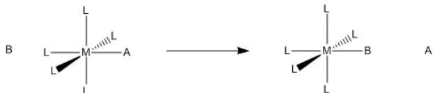
Figure 3.1.1: Substitution of one ligand for another in a coordination complex.
