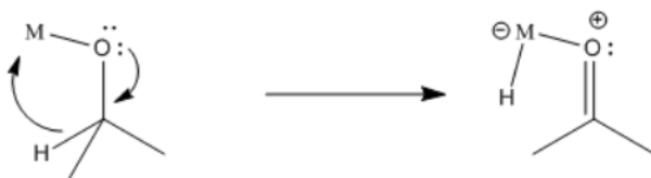
Figure 4.4.4: The reverse of a 1,2-addition is a 1,2-elimination.
