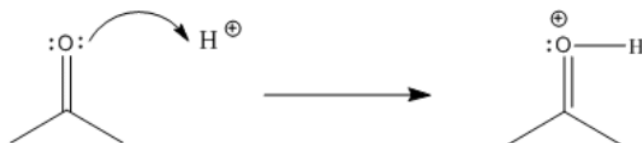
Figure 3.4.1: Activation of a carbonyl via donation to a proton.
