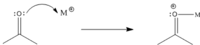
Figure 4.4.1: Activation of an organic carbonyl by a metal ion.
