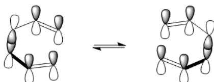
Figure 10.2.4: Orbital rearrangement in a Cope rearrangement
