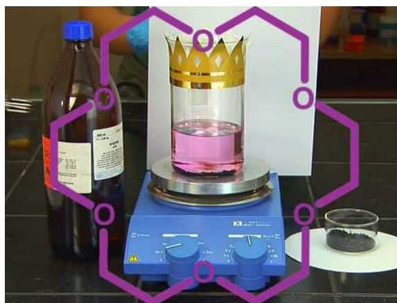
Figure 9.2.6. Effect of a Crown Ether on the Solubility of \text{KMnO}_4 in Benzene. Normally which is intensely purple, is completely insoluble in benzene which has a relatively low dielectric constant. In the presence of a small amount of crown ether, \text{KMnO}_4 dissolves in benzene as shown by the reddish purple color caused by the permanganate ions in solution. Video from Chem Toddler
