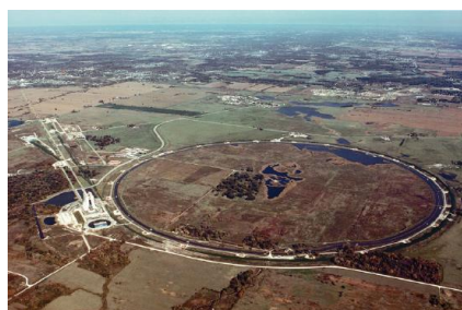
Figure 18.2.7 A Synchrotron An aerial photograph of what is currently the world's most powerful particle accelerator, the Tevatron at the Fermi National Accelerator Laboratory (Fermilab) in Illinois. The large tube characteristic of a synchrotron is 4 miles in circumference, contains 1000 superconducting magnets cooled by liquid helium, and can accelerate a beam of protons to almost the speed of light, giving them an energy greater than 1 TeV (teraelectronvolt = 10^3 GeV = 10^{12} eV) for collisions with other particles.
