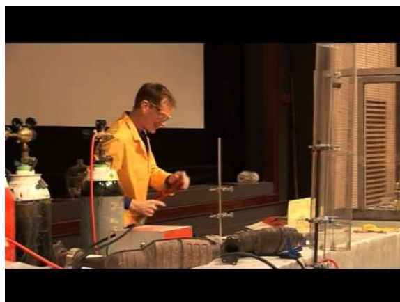
Figure 13.1.3 Burning flour dust A pile of flour is only scorched by a flame, but when the same flour is sprayed into the flame, it burns rapidly. Peter Wolthers has a series of videos demonstrating combustion reactions that you can watch
