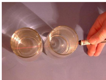
Figure 9.6.1 Tyndall Effect, the Scattering of Light by Colloids The glass on the left has dilute colloidal silver, the one on the right tap water. The red laser pointer beam is scattered by the Tyndall effect in the glass on the left.
