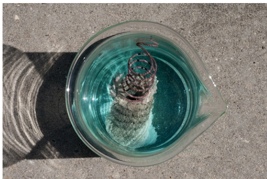
Figure 12.7.2 The Single-Displacement Reaction of Metallic Copper with a Solution of Silver Nitrate When a copper coil is placed in a solution of silver nitrate, silver ions are reduced to metallic silver on the copper surface, and some of the copper metal
