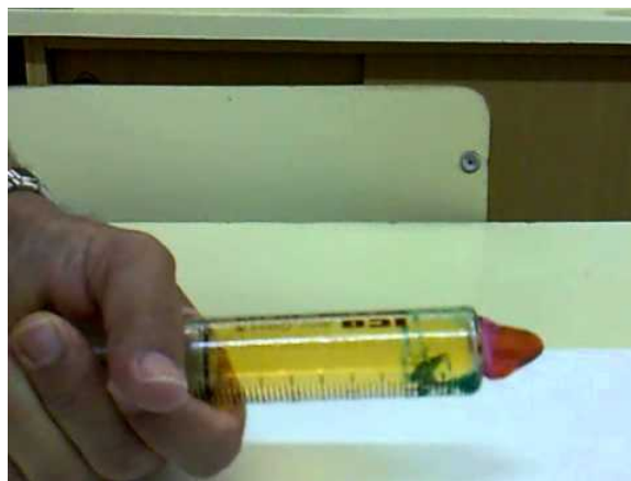
Figure 14.5.3 The Effect of Changing the Volume (and Thus the Pressure) of an Equilibrium Mixture of N_2O_4 and NO_2 at Constant Temperature (a) The syringe with a total volume of 15 mL contains an equilibrium mixture of N_2O_4 and NO_2 ; the red-brown color is proportional to the NO_2 concentration. (b) If the volume is rapidly decreased by a factor of 2 to 7.5 mL, the initial effect is to double the concentrations of all species present, including NO_2 . Hence the color becomes more intense. (c) With time, the system adjusts its composition in response to the stress as predicted by Le Châtelier's principle, forming colorless N_2O_4 at the expense of red-brown NO_2 , which decreases the intensity of the color of the mixture. Video from joan-ramon i pinazo
