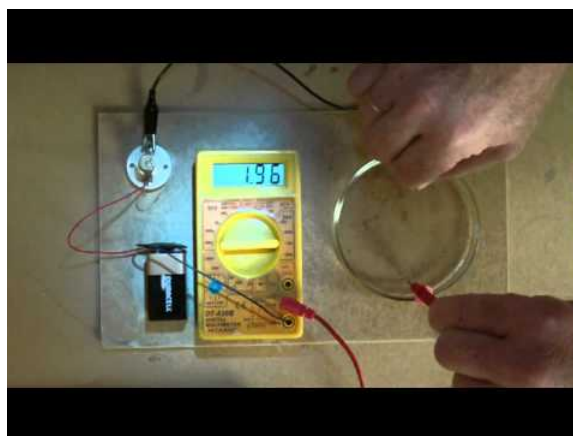
Figure 9.1.4 The Effect of Ions on the Electrical Conductivity of Water An electrical current will flow and light the bulb only if the solution contains ions. (a) Deionized or distilled water or an aqueous solution of a nonelectrolyte allows almost no current to flow. (b) A weak electrolyte such as tap or river water produces a few ions, allowing some current to flow. (c) A strong electrolyte formed by adding salt produces many ions, allowing more current to flow. Video from MDR Science Academy
