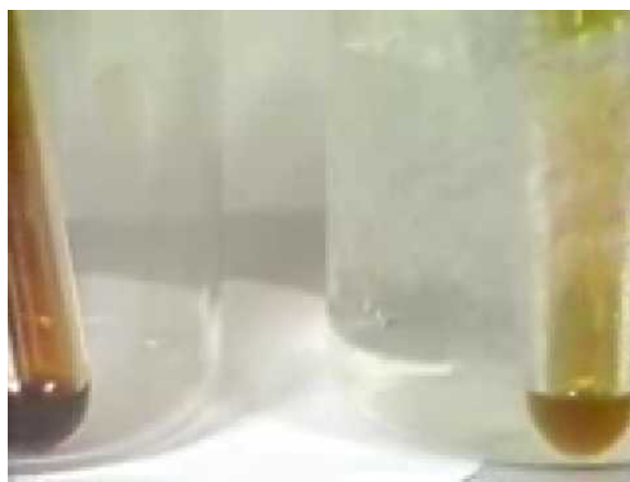
Figure 14.1.1 The \text{N}_2\text{O}_4(\text{g}) \rightleftharpoons 2\text{NO}_2(\text{g}) System at Different Temperatures At room temperature a mixture of gaseous \text{N}_2\text{O}_4 and \text{NO}_2 is present. If the sample is placed in a warm bath, the equilibrium shifts to the right and \text{NO}_2 predominates as shown by the redder color. If it is placed in an ice bath the equilibrium shifts to the left and colorless \text{N}_2\text{O}_4 predominates. The composition of the mixture and hence the color do not change further with time once the system reaches equilibrium at the new temperature. At dry ice temperature ( -78.4^\circ\text{C} ), the system would contain essentially pure solid \text{N}_2\text{O}_4 , which is colorless. The video is from NuclearRabbit on YouTube
