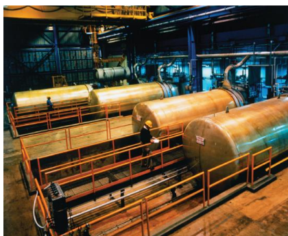
Figure 6.6.6 A Portion of a Plant for Separating Uranium Isotopes by Effusion of \text{UF}_6 The large cylindrical objects (note the human for scale) are so-called diffuser (actually effuser) units, in which gaseous \text{UF}_6 is pumped through a porous barrier to partially separate the isotopes. The \text{UF}_6 must be passed through multiple units to become substantially enriched in ^{235}\text{U} . While gaseous diffusion was the original method of uranium isotope separation today, this process is done using centrifuges
