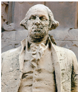
Figure 12.6.2 Acid Rain Damage to a Statue of George Washington Both marble and limestone consist of \text{CaCO}_3 , which reacts with acid rain in an acid–base reaction to produce \text{CaSO}_4 . Because \text{CaSO}_4 is somewhat soluble in water, significant damage to the structure can result.
