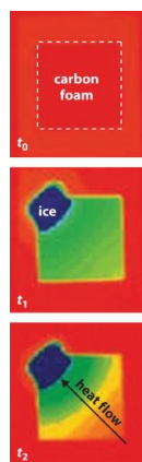
Figure 16.1.5 Thermograms Showing That Heat Is Absorbed from the Surroundings When Ice Melts at 0°C By convention, a thermogram shows cold regions in blue, warm regions in red, and thermally intermediate regions in green. When an ice cube (the system, dark blue) is placed on the corner of a square sample of low-density carbon foam with very high thermal conductivity, the temperature of the foam is lowered (going from red to green). As the ice melts, a temperature gradient appears, ranging from warm to very cold. An arrow indicates the direction of heat flow from the surroundings (red and green) to the ice cube. The amount of heat lost by the surroundings is the same as the amount gained by the ice, so the entropy of the universe does not change.
