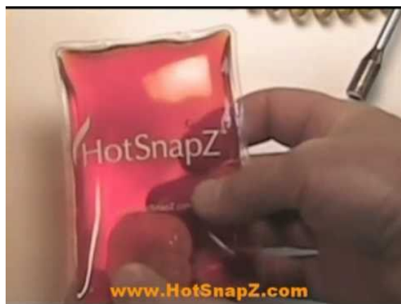
Figure 15.6.2 An Instant Hot Pack Based on the Crystallization of Sodium Acetate The hot pack is at room temperature prior to agitation (left). Because the sodium acetate is in solution, you can see the metal disc inside the pack. After the hot pack has been agitated, the sodium acetate crystallizes (right) to release heat. Because of the mass of white sodium acetate that has crystallized, the metal disc is no longer visible.
