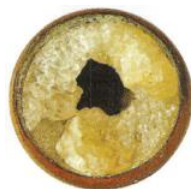
Figure 9.4.3 Boiler Scale in a Water Pipe Calcium carbonate (CaCO 3 ) deposits in hot water pipes can significantly reduce pipe capacity. These deposits, called boiler scale, form when dissolved CO 2 is driven into the gas phase at high temperatures.
