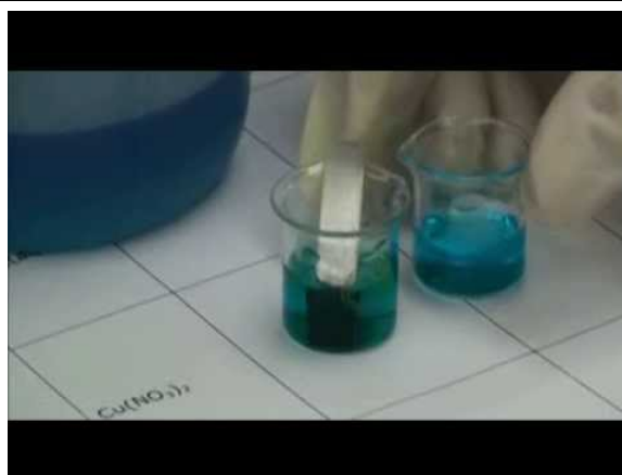
Figure 17.1.2 The Reaction of Metallic Zinc with Aqueous Copper(II) Ions in a Single Compartment When a zinc plate is inserted into a beaker that contains an aqueous solution of copper(II) sulfate, a spontaneous redox reaction occurs: the zinc electrode dissolves to give \text{Zn}^{2+}(\text{aq}) ions, while \text{Cu}^{2+}(\text{aq}) ions are simultaneously reduced to metallic copper. The reaction occurs so rapidly that the copper is deposited as very fine particles that appear black, rather than the usual reddish color of copper. Video from CMUChemVideos
