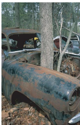
Figure 12.7.1 Rust Formation The corrosion process involves an oxidation–reduction reaction in which metallic iron is converted to \text{Fe}(\text{OH})_3 , a reddish-brown solid.
