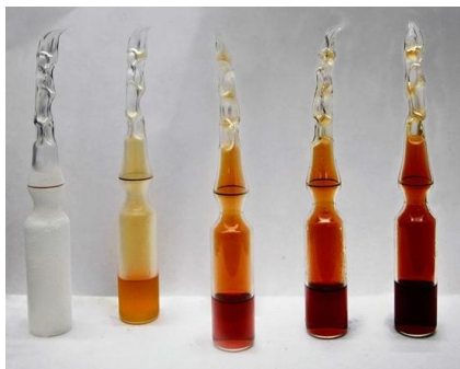
Figure 14.5.4 The Effect of Temperature on the Equilibrium between Gaseous N_2O_4 and NO_2 The value of K changes with temperature of the same 99.9% pure NO_2/N_2O_4 sealed in an ampoule. From left to right -196^\circ \text{C} , 0^\circ \text{C} , 23^\circ \text{C} , 35^\circ \text{C} , 50^\circ \text{C} . In the endothermic reaction, the equilibrium position can be shifted by changing the temperature. When heat is added and the temperature increases, the reaction shifts to the right and the flask turns reddish brown due to an increase in NO_2 . When heat is removed and the temperature decreases, the reaction shifts to the left and flask turns colorless due to an increase in N_2O_4 . This demonstrates Le Chatelier's Principle because the equilibrium shifts in the direction that consumes energy. Figure used with permission from Wikipedia.
