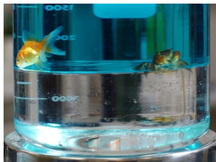
Figure 9.2.3 Water is immiscible with with perfluoroheptane (and most halogenated compounds). Because water is less dense than the perfluoroheptane, the water layer floats on top. The goldfish is swimming in the water layer. Figure from the Wikipedia ..
