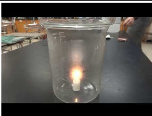
Figure 11.3.3 An Example of a Combustion Reaction The wax in a candle is a high-molecular-mass hydrocarbon, which produces gaseous carbon dioxide and water vapor in a combustion reaction. When the candle is allowed to burn inside a flask, drops of water, one of the products of combustion, form which we can verify using cobalt chloride test paper. We can demonstrate that carbon dioxide is a product by precipitating calcium carbonate from limewater..
