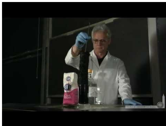
Figure 13.1.1 The Effect of Concentration on Reaction Rates Mixing sucrose with dilute sulfuric acid in a beaker (a, right) produces a simple solution. Mixing the same amount of sucrose with concentrated sulfuric acid results in a dramatic reaction that eventually produces a column of black porous graphite (c) and an intense smell of burning sugar. Video from UC Berkeley
