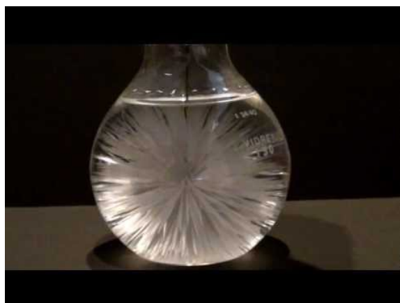
Figure 9.2.2 Crystallization of Sodium Acetate out of a Supersaturated Solution: The crystallization of sodium acetate out of a supersaturated solution can be spectacular. In this video from Mike Shin a small seed crystal is introduced into the middle of the solution
