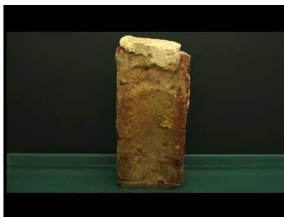
Figure 7.3.4 The Phenomenon of Capillary Action: Water rises through a brick in a time lapse video
