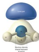
Figure 5.1.4 The Difference in the Space Occupied by a Lone Pair of Electrons and by a Bonding Pair As with SO_2 , this composite model of electron distribution and negative electrostatic potential in ammonia shows that a lone pair of electrons occupies a larger region of space around the nitrogen atom than does a bonding pair of electrons that is shared with a hydrogen atom.
