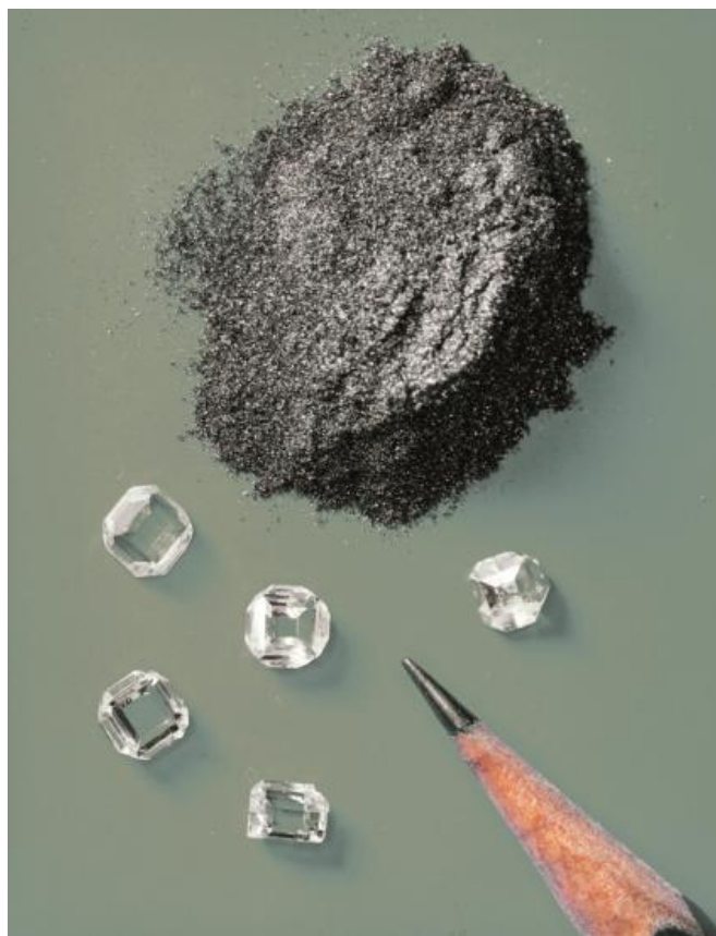
Figure 15.5.1 Elemental Carbon Although graphite and diamond are both forms of elemental carbon, graphite is more stable at 1 atm pressure and 25°C than diamond is. Given enough time, diamond will revert to graphite under these conditions. Hence graphite is the standard state of carbon.
