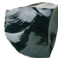
Figure 8.1.1 Cleaving a Crystal of an Ionic Compound along a Plane of Ions Deformation of the ionic crystal causes one plane of atoms to slide along another. The resulting repulsive interactions between ions with like charges cause the layers to separate.
