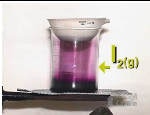
Figure 7.5.2 The Sublimation of Solid Iodine When solid iodine is heated at ordinary atmospheric pressure, it sublimates. When the I 2 vapor comes in contact with a cold surface, it deposits I 2 crystals.
