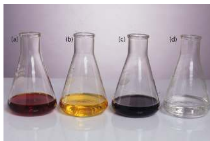
Figure 9.41 Endpoint for the determination of the total chlorine residual. (a) Acidifying the sample and adding KI forms a brown solution of I_3^- . (b) Titrating with Na_2S_2O_3 converts I_3^- to I^- with the solution fading to a pale yellow color as we approach the end point. (c) Adding starch forms the deep purple starch- I_3^- complex. (d) As the titration continues, the end point is a sharp transition from a purple to a colorless solution. The change in color from (c) to (d) typically takes 1–2 drops of titrant.
