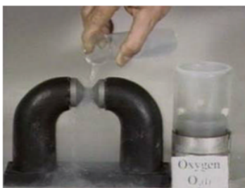
Figure 1.11.5. Demonstration showing blue liquid O_2 attracted to the poles of a permanent magnet. From jchemed.chem.wisc.edu/jcesoft.../PARANIO/9.HTM
