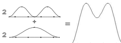
Figure 4. Pi-electron density in butadiene.
