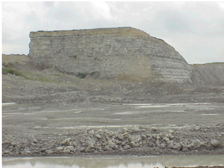
Figure 4.2.4.27: Limestone quarry formation, showing the 45° ripping technique (Copyright Halliburton Energy Services).
