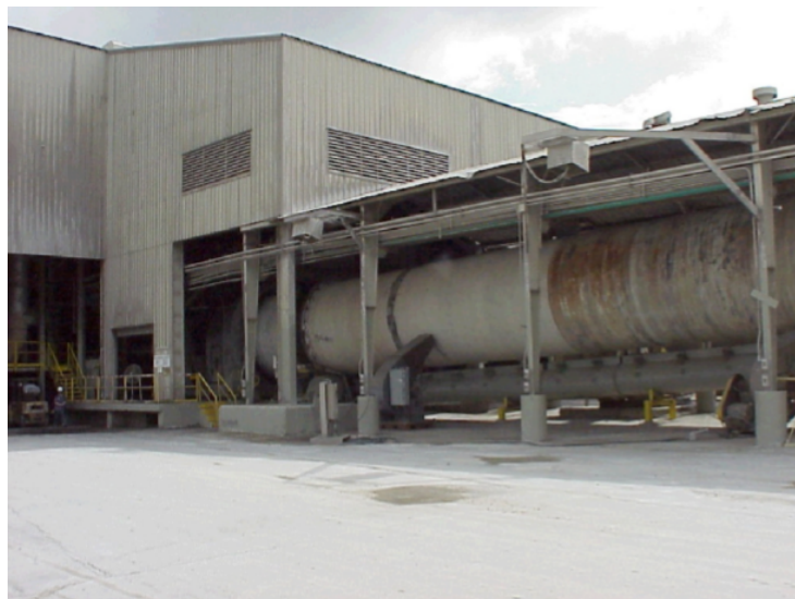
Figure 4.2.4.35: A wet rotary kiln (Copyright Halliburton Energy Services).
