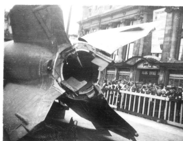
Figure 7.2.10: View of the V-2 rocket showing the graphite vanes for directional control.
