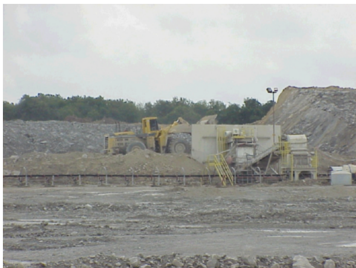
Figure 4.2.4.28: Mobile crusher and XRF unit (Copyright Halliburton Energy Services).
