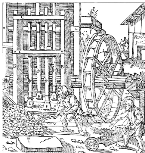
Figure 9.3.7: The cam principle as applied to a rock-crushing mill illustrated by Georgius Agricola in his book De Re Metallica (1556).
