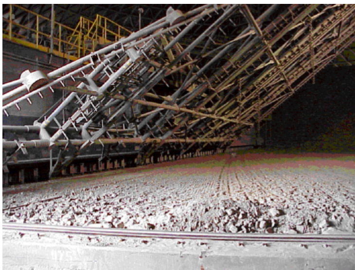
Figure 4.2.4.32: Raking device for reclaiming stored limestone (Copyright Halliburton Energy Services).
