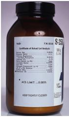
Figure 7.1.1. Certificate of analysis for a production lot of NaBr. The result for iron meets the ACS specifications, but the result for potassium does not.
