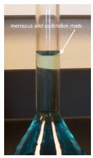
Figure 2.4.7: Proper position of the solution's meniscus relative to the volumetric flask's calibration mark.
