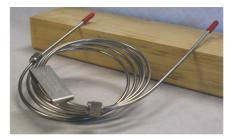
Figure 12.4.2. Typical example of a packed column for gas chromatography. This column is made from stainless steel and is 2 m long with an internal diameter of 3.2 mm. The packing material in this column has a particle diameter of 149–177  $\mu$ m. To put this in perspective, beach sand has a typical diameter of 700  $\mu$ m and the diameter of fine grained sand is 250  $\mu$ m.
