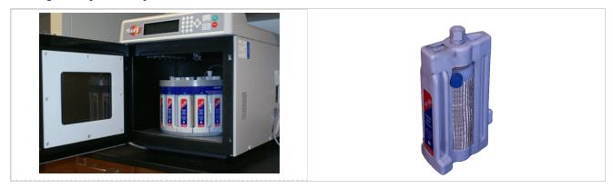
Figure 7.3.7. Microwave digestion unit: on the left is a view of the unit's interior showing the carousel that holds the digestion vessels; on the right is a close-up of a Teflon digestion vessel, which is encased in a thermal sleeve. The pressure relief value, which is part of the vessel's blue cap, contains a membrane that ruptures if the internal pressure becomes too high.
