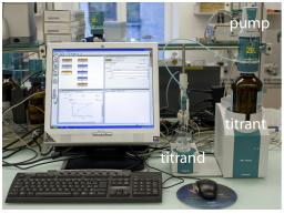
Figure 9.1.5. Typical instrumentation for an automated acid—base titration showing the titrant, the pump, and the titrand. The pH electrode in the titrand's solution is used to monitor the titration's progress. You can see the titration curve in the lower-left quadrant of the computer's display. Modified from: Datamax (commons. wikipedia.org).
