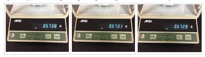
**Figure 2.1.1:** When weighing an sample on a balance, the measurement fluctuates in the final decimal place. We record this sample's mass as  $0.5730 \text{ g} \pm 0.0001 \text{ g}$ .
