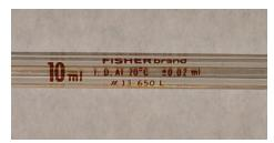
Figure 2.4.6: Close-up of the 10-mL transfer pipet from Figure 2.4.3.
