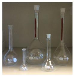
Figure 2.4.5: A collection of volumetric flasks with volumes of 10 mL, 50 mL, 100, mL, 250 mL, and 500 mL.
