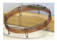
Figure 12.4.3. Typical example of a capillary column for gas chromatography. This column is 30 m long with an internal diameter of 247 µm. The interior surface of the capillary has a 0.25 µm coating of the liquid phase.
