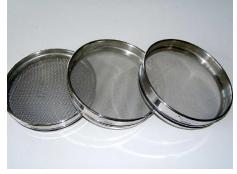
Figure 8.4.1. Three sieves with, from left to right, mesh sizes of 1700  $\mu$ m, 500  $\mu$ m, and 250  $\mu$ m. Source: BMK (commons.wikimedia.com).
