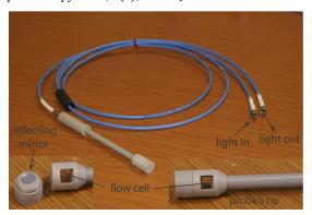
Figure 10.3.7. Example of a fiber-optic probe. The inset photographs at the bottom of the figure provide close-up views of the probe's flow cell and the reflecting mirror.
