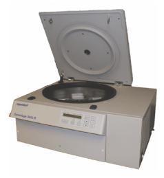
Figure 7.6.3. Bench-top centrifuge capable of reaching speeds up to 14000 rpm and centrifugal forces of  $20800 \times g$ . This particular centrifuge is refrigerated, allowing samples to be cooled to temperatures as low as  $-4^{\circ}$ C.
