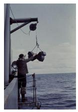
Figure 7.3.2. Bottom grab sampler being prepared for deployment. Source: NOAA.
