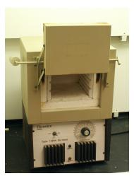
Figure 2.4.8: Example of a muffle furnace.
