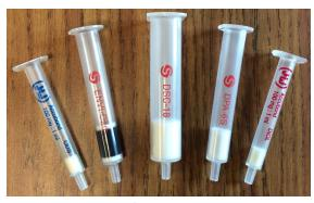
Figure 7.6.10. Selection of solid phase extraction cartridges for liquid samples. The solid adsorbent is the white or black material in each cartridge. From left-to-right, the absorbent materials are octadecylsilane, carbon, octadecylsilane, polyamide resin, and diol; see Table 7.6.5 for additional details. The size of the cartridges dictates the volume of sample used; from left-to-right, these cartridges use samples of 1 mL, 3 mL, 6 mL, 3 mL, and 1 mL.
