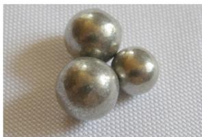
Figure *[Math Processing Error]*: Ni(CO)<sub>4</sub> spheres prepared through the Mond process (René Rausch, [Nickel kugeln](#), [CC BY-SA 3.0 DE](#))
