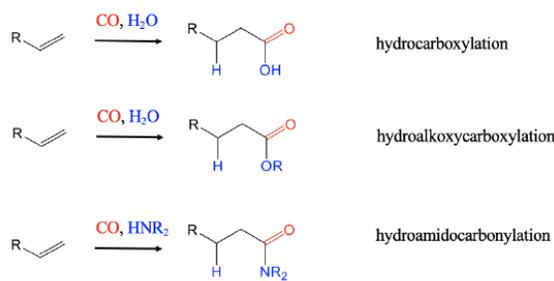
Figure 12.2.6 Hydrocarbonylation reactions
