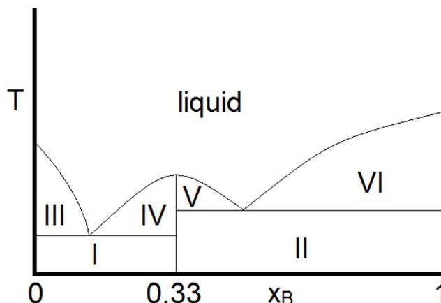
Figure 27.1.3: A simplified phase diagram of a two-component system that exhibits an eutectic point.
