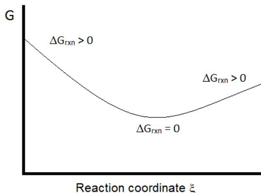
From the diagram above, it should be clear that the direction of spontaneous change is determined by minimizing
