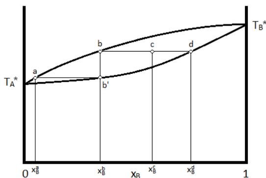
Figure 25.3.2: A typical temperature vs. composition diagram.
