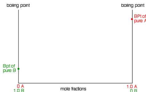
For mixtures of A and B, you might perhaps have expected that their boiling points would form a straight line joining the two points we've already got. Not so! In fact, it turns out to be a curve.
