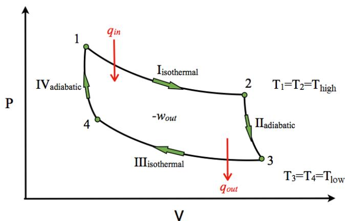
Figure 13.1.2: A P-V diagram of the Carnot Cycle.
