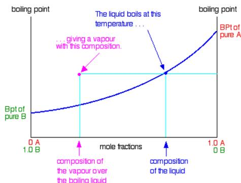
The diagram just shows what happens if you boil a particular mixture of A and B. Notice that the vapor over the top of the boiling liquid has a composition which is much richer in B - the more volatile component. If you repeat this exercise with liquid mixtures of lots of different compositions, you can plot a second curve - a vapor composition line.
