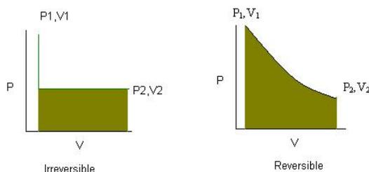
The graphs clearly show work done (area under the curve) is greater in a reversible process.
