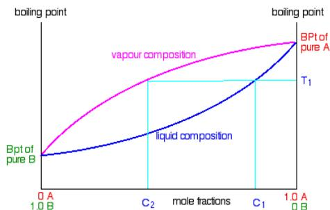
All you have to do is to use the liquid composition curve to find the boiling point of the liquid, and then look at what the vapor composition would be at that temperature. Notice again that the vapor is much richer in the more volatile component B than the original liquid mixture was.
