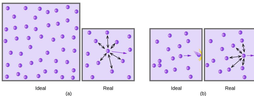
Figure 1.1.3: (a) Attractions between gas molecules serve to decrease the gas volume at constant pressure compared to an ideal gas whose molecules experience no attractive forces. (b) These attractive forces will decrease the force of collisions between the molecules and container walls, therefore reducing the pressure exerted compared to an ideal gas.
