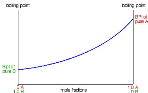
To make this diagram really useful (and finally get to the phase diagram we've been heading towards), we are going to add another line. This second line will show the composition of the vapor over the top of any particular boiling liquid.
