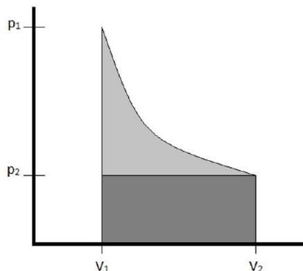
The work is depicted as the shaded portion of the graph. It is clear to see that the reversible expansion (the work for which is shaded in both light and dark gray) exceeds that of the irreversible expansion (shaded in dark gray only) due to the changing pressure of the reversible expansion. In general, it will always be the case that the work generated by a reversible pathway connecting initial and final states will be the maximum work possible for the expansion.
