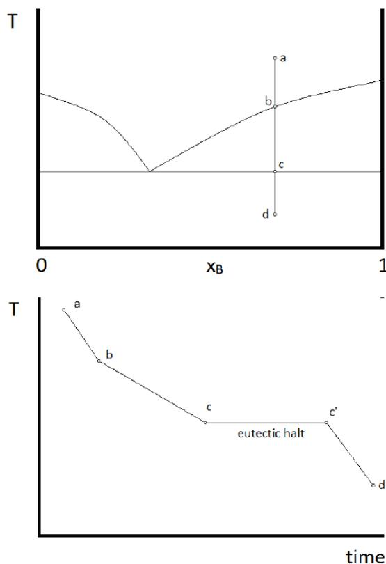
Figure 27.2.1: (A) cooling of a two-component system from liquid to solid. (B) Cooresponding cooling curve for this process.
