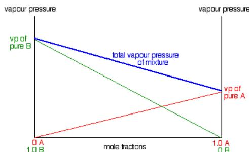
We're going to convert this into a boiling point / composition diagram. We'll start with the boiling points of pure A and B. Since B has the higher vapor pressure, it will have the lower boiling point. If that is not obvious to you, go back and read the last section again!
