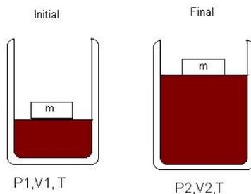
This shows the expansion of gas at constant temperature against weight of an object's mass ( $m$ ) on the piston. Temperature is held constant, therefore the change in energy is zero ( $U=0$ ). So, the heat absorbed by the gas equals the work done by the ideal gas on its surroundings. Enthalpy change is also equal to zero because the change in energy zero and the pressure and volume is constant.
