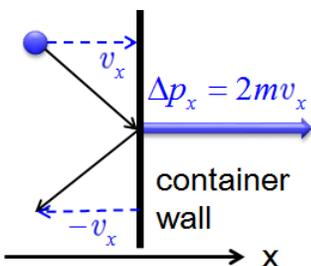
Figure 2.1.2: Momentum transfer (impulse) from a molecule to the container wall as it bounces off the wall.  $v_x$  and  $\Delta p_x$  are the  $x$  component of the molecular velocity and the momentum transferred to the wall, respectively. The wall is perpendicular to  $x$  axis. Since the collisions are elastic, the molecule bounces back with the same velocity in the opposite direction.
