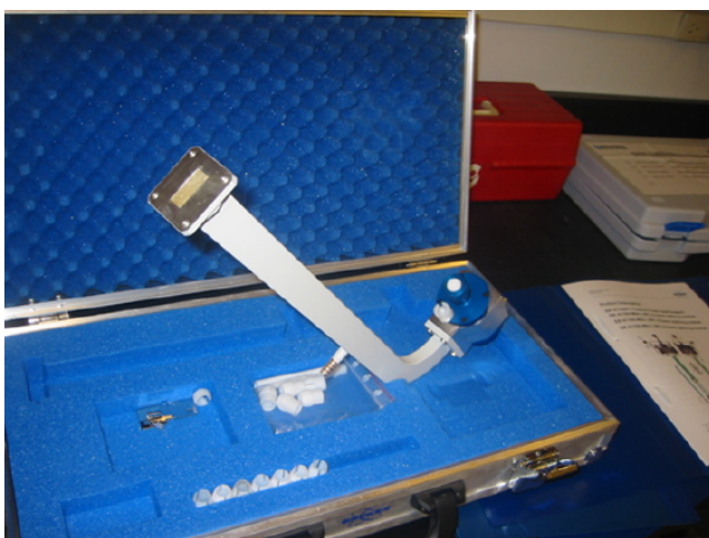
Figure 5.15.2: Microwave waveguides direct microwaves through the EPR instrument. The optical analog would be a fiber optic.
