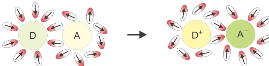
Figure 1: Changes in solute-solvent interactions lead to solvatochromic shifts in absorption and fluorescence spectra of the same fluorophore. (CC BY-SA-NC; Andrei Tokmakoff)
