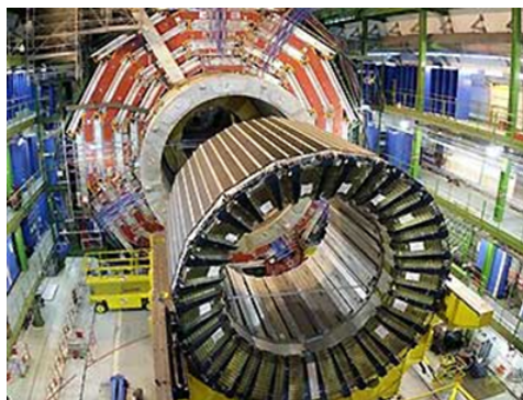
Right: Magnet core of the largest superconducting solenoid magnet at European Organization for Nuclear Research's Large Hadron Collider.
