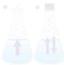
Figure 13.2.2: The water in an open contain will eventually disappear as it evaporates (A). In a closed container, the rate of evaporation equals the rate of condensation (B).
