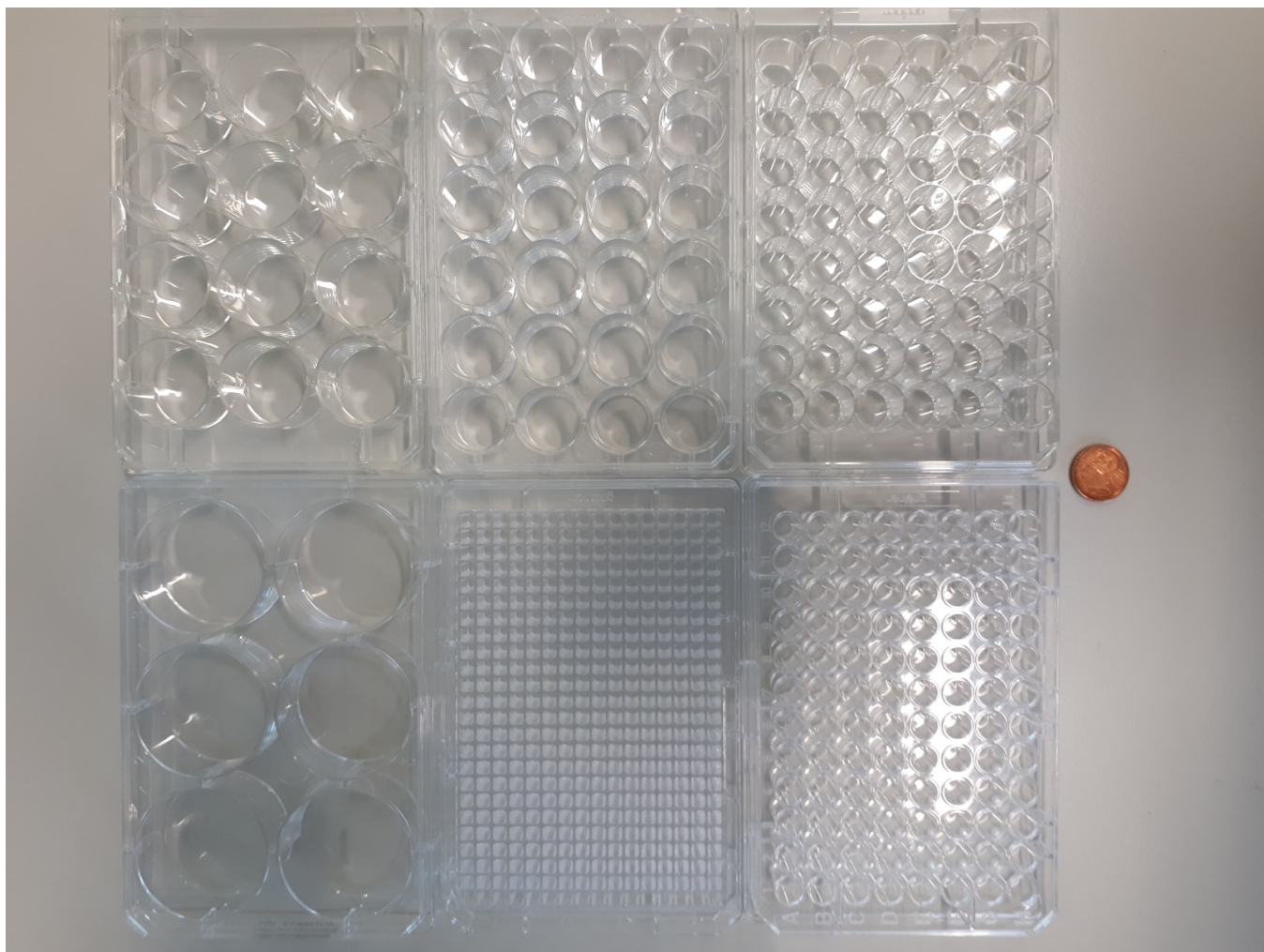
Figure 1: Six different microtiter well-plates, consisting of multiple small-volume test containers. In clockwise direction starting from the LOWER left: 6-wells plate, 12-wells plate, 24-wells plate, 48-wells plate, 96 wells plate, 384 wells plate.
