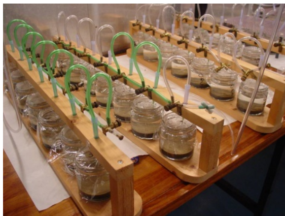
Figure 1. Experimental design of a chronic sediment toxicity experiment, showing the experimental units and the aeration system.
