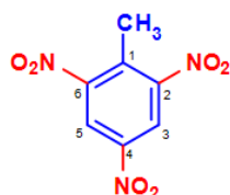
Figure 17. 2,4,6-Trinitrotoluene, or TNT , a common explosive used for both industrial and military purposes, is consisted of a toluene base (labeled in blue), along with three nitro groups attached as substituents (labeled in red). The explosive is characteristic for its resistance to external shock and friction, making it useful in many applications where other highly sensitive explosives would simultaneously detonate.
